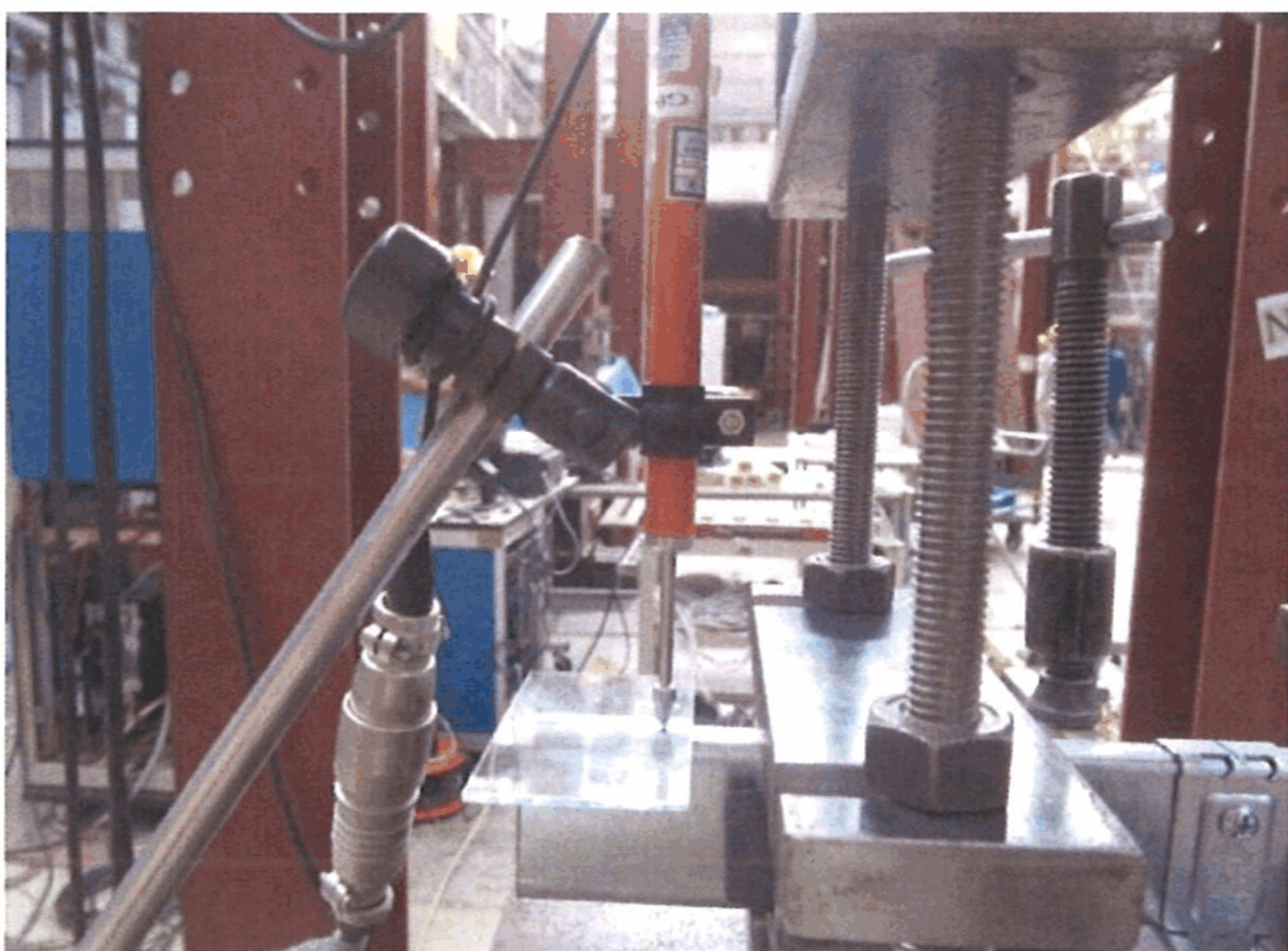
(c) 変位計の設置状況(D.T.1)
