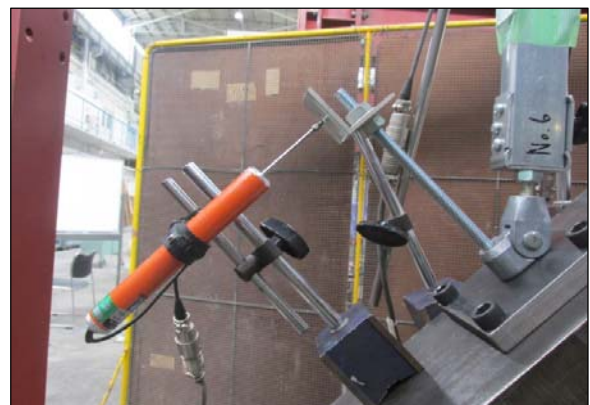
(f) 変位計の設置状況 (D.T.3)
