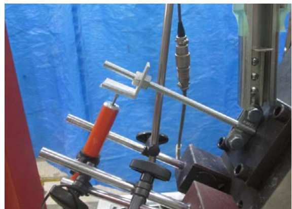
(f) 変位計の設置状況 (D.T.3)
